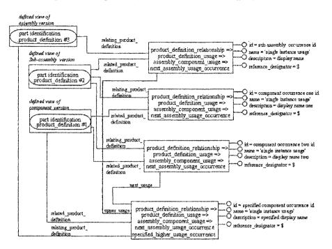
Fig. 1. Multi-level assembly DMU instance diagram in the PDM schema.
