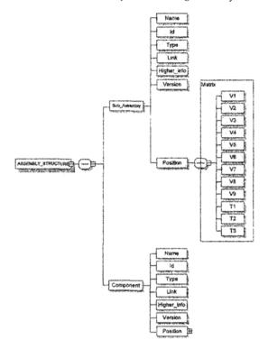
Fig. 2. XML schema structure for assembly.
